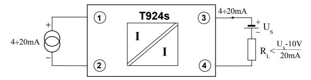
Load resistance,  $R_L$ , is limited by the supply voltage,  $U_S$ , according to the formula presented in the above drawing. If necessary, the supply voltage may be increased up to 36V.
