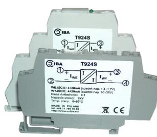
Separator provides galvanic isolation between input and output current loops while preserving the signal with basic accuracy better than 0.1%. Factory test isolation voltage equals 2kV.
