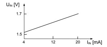
Output: current 4÷20 mA voltage drop at output terminals 10÷36V
