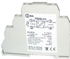
T924s-PS is a passive separator of 4÷20mA signal (in fact, separator operates linearly from 2.5mA to about 25mA where internal limiting circuit turns on). Factory test isolation voltage equals 2kV.
