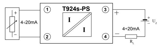
Acceptable voltage drop at separator's output may be as high as 28V but, assuming standard supply voltage  $U_z$ =24V, accounting for 4V internal drop and typical load resistance,  $R_L$ =50 $\Omega$ , there is still about 19V left for the transmitter supply (at  $I_{IN}$ = $I_{OUT}$ =20mA).
