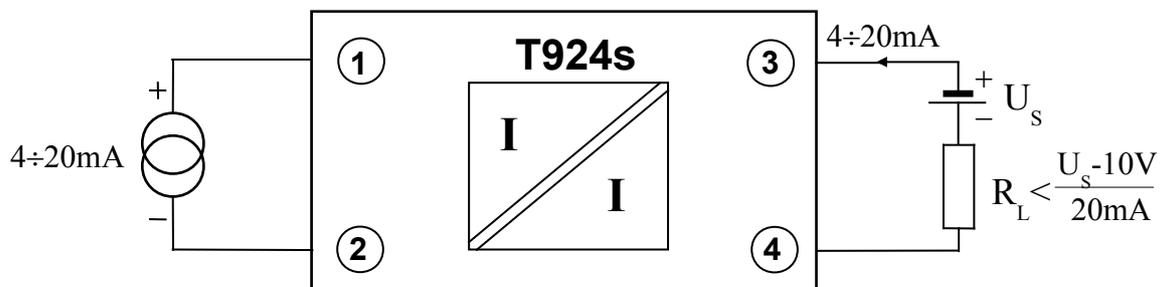
Load resistance,  $R_L$ , is limited by the supply voltage,  $U_s$ , according to the formula presented in the above drawing. If necessary, the supply voltage may be increased up to 36V.
