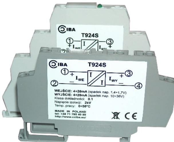
Separator provides galvanic isolation between input and output current loops while preserving the signal with basic accuracy better than 0.1%. Factory test isolation voltage equals 2kV.
