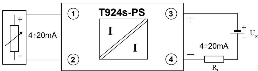
Acceptable voltage drop at separator's output may be as high as 28V but, assuming standard supply voltage  $U_Z=24V$ , accounting for 4V internal drop and typical load resistance,  $R_L=50\Omega$ , there is still about 19V left for the transmitter supply (at  $I_{IN}=I_{OUT}=20mA$ ).
