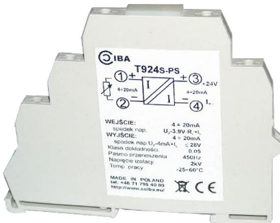
T924s-PS is a passive separator of 4÷20mA signal (in fact, separator operates linearly from 2.5mA to about 25mA where internal limiting circuit turns on). Factory test isolation voltage equals 2kV.
