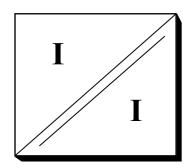
Module T924p3 contains three independent and isolated passive separators of  $4\div20mA$  signal (in fact separators function from almost 0mA to about 25mA where internal limiting circuit turns on). Factory test isolation voltage equals 2kV.
