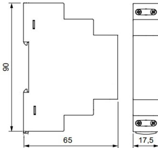
Module T924P1 is a passive separator of 4÷20mA signal (it functions in fact from almost 0mA to about 25mA where internal limiting circuit turns on). Factory test isolation voltage equals 2kV.
