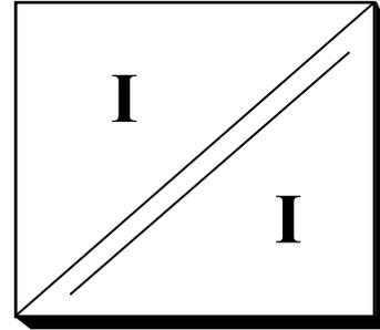
T924PS1 is a passive separator of 4÷20mA signal (in fact, separator operates linearly from 2.5mA to about 25mA where internal limiting circuit turns on). Factory test isolation voltage equals 2.5kVrms.
