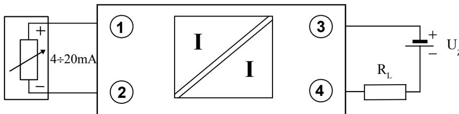
One of the main advantages of the module is a system of overvoltage and overcurrent protections preventing accidental damage during installation or malfunction of other automation elements during exploitation. Both input and output are protected against overvoltage and bias reversal. The input current is limited internally to ca. 25mA which is rare in passive separators. Absolute maximum ratings are listed at the end of the data sheet.
